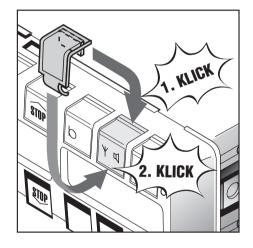
Keys that have no function due to the roof configuration are "clipped" (with black or transparent clips) after coding to block them mechanically.
