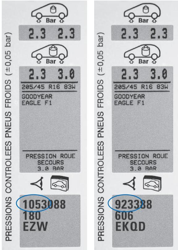
The RP number (Orga) is in the bottom half of the vehicle data label. The last two digits of the number are irrelevant as far as looking for the spare part is concerned.
