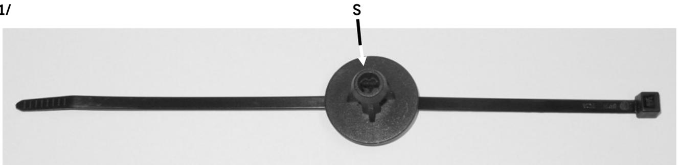
Remove original ABS clips and fit ABS wire and/ or sensor bracket strain-free by using cable clips (pic 1) delivered by Bilstein.
