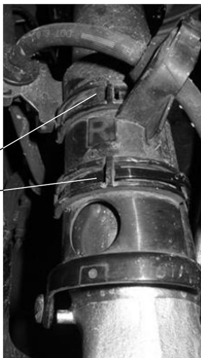
Fixing of original brake hose holder (plastic) by using both cable strips (B) delivered by BILSTEIN, same as original.
