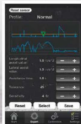
The customer can make the adjustments he wants to the regulation of the vertical acceleration (up-and-down movement), horizontal acceleration (transverse acceleration to the left and right) and longitudinal acceleration (accelerating and braking) through his iPhone.
