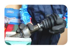
1. Put the short boot clamp on the shaft. Slide the boot on the shaft.
