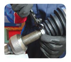
5. Fit the short clamp onto the CV-boot and tighten it with a suitable tool. Pull the boot onto the CV-joint.
