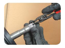
4. Expand and remove the circlip with circlip removal pliers.
