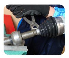
2. Place the driveshaft in a vice (with aluminum or protective jaws).
