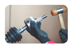
3. Press the new CV-joint onto the shaft. Tap with a rubber hammer until the circlip locks into its groove in the inner race of the CV-joint. Remove the hose clip.
