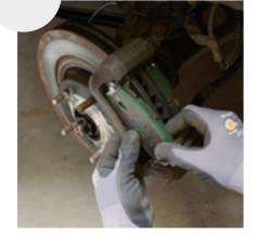
2. Release the brake calliper and remove the brake pads. Attention: when replacing brake discs, always replace the brake pads with them and replace all brake discs/brake pads on the respective axle!
