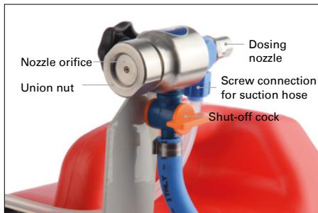
\* Dosing nozzles have a defined bore to permit a fixed agent throughput. The throughput can be altered as required by fitting a nozzle of a different size.
