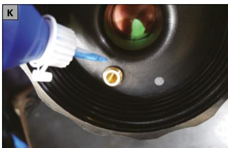
Apply thread lock adhesive to the nut and then tighten it.
