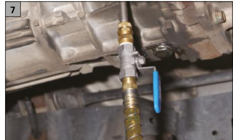
8. Activate the liquid control valve at the end of the PVC hose (Fig. 8).
