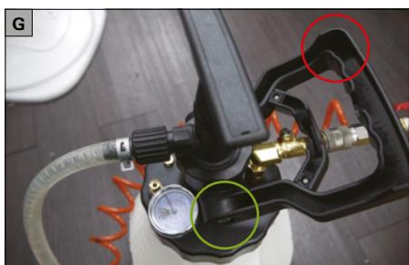
Discharge the pressure in the tank after deactivating the air valve by pulling the square handle on the tank lid (F to G). The pressure discharge valve (green marking in Fig. G) discharges pressure and makes a distinctive noise.
