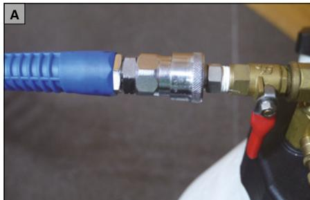
Connect the workshop compressed air supply to the tank (A) and operate the air valve to activate and deactivate the air supply.
