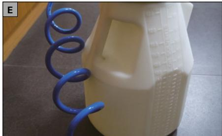
Check for evidence of leaks in the tank (E) while pressure in the tank is accumulating.
