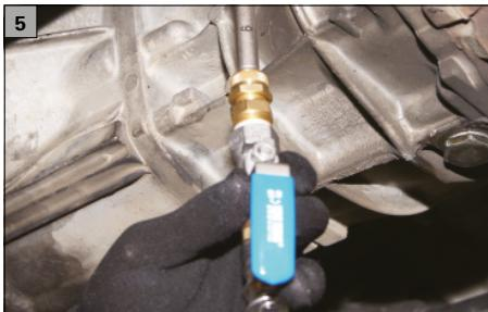
6. Fill the 12.5 l (3.3 gal) tank with the quantity of ATF fluid required in each case.
