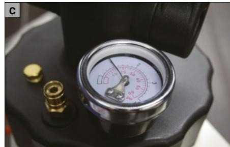
Check whether the manometer gauge on the lid of the tank moves when the pressure in the tank increases (C).
