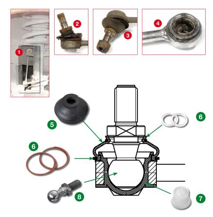
other parts caused by an accident or bumps can cause damage to the rubber bellows and lead to a premature failure of the connecting rod. While fitting, always follow the manufacturers' installation instructions.
