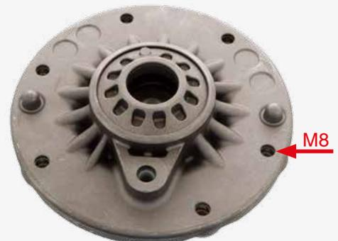
Various strut mountings which differ in the number of holes and thread have been fitted in the series referred to above.
