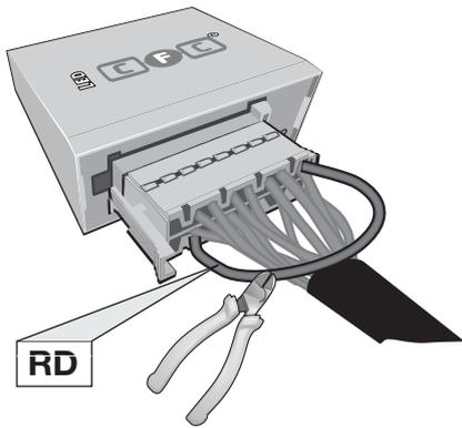
Pin 11 and Pin 2 disconnected
