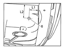
L1 = 85 mm from hole (6) to edge of spare tire recess
