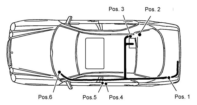
The routing of the wiring harness shown above is identical on the W 210 Sedan and S 210 T-model (station wagon)!
