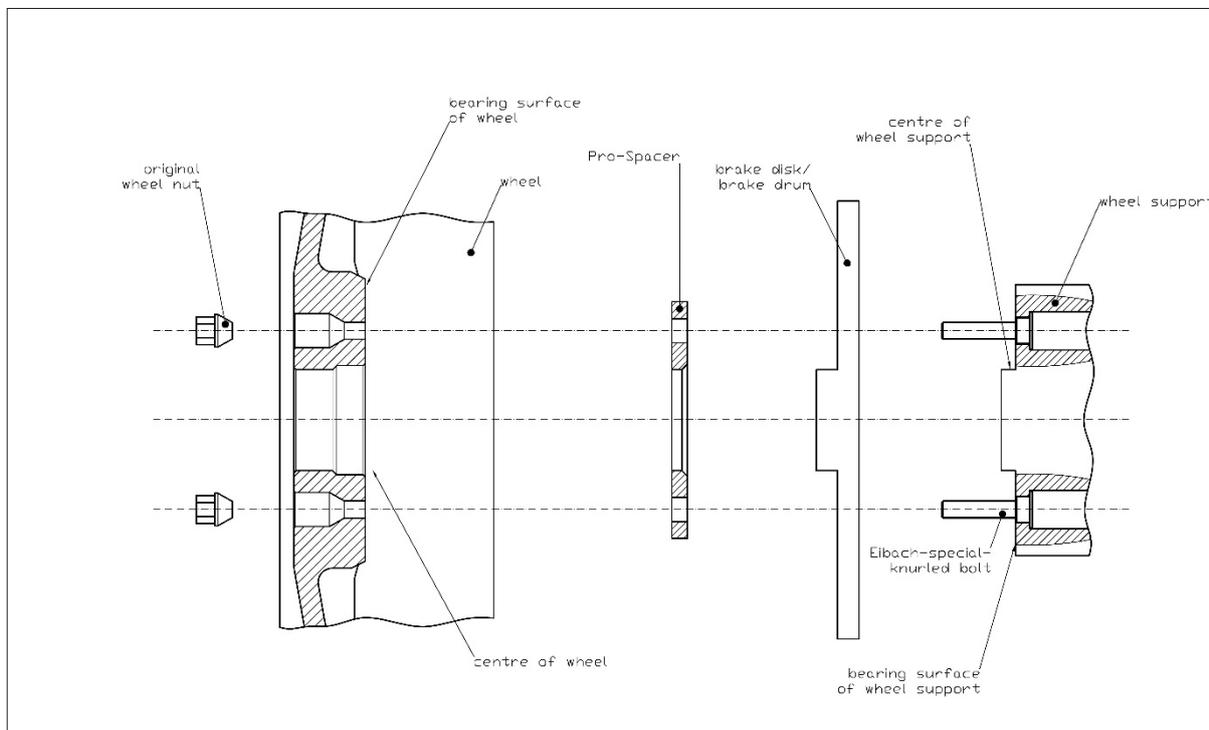
1. The center alignments and bearing surfaces of the wheel support and the wheel (Figure 1) must be free of rust and dirt and clean. Use a wire brush for this purpose and proceed with caution, to avoid damaging other components.
