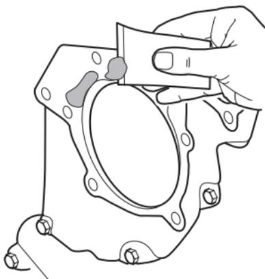
**EN** Only fit water pump with gasket(s) supplied with it. Do not use silicone sealants unless recommended by the manufacturer. Observe manufacturer`s installation specifications.
