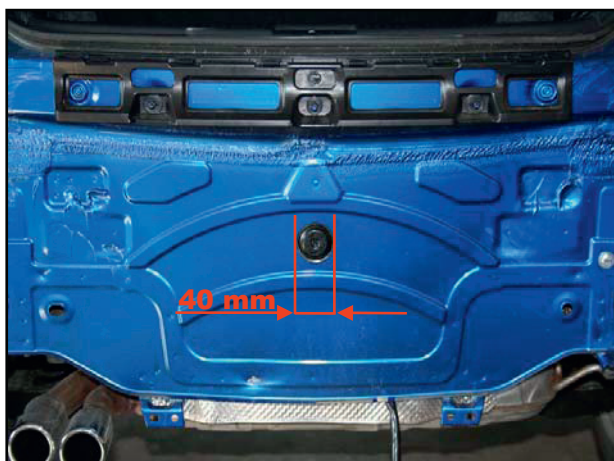
Loch Ø 40 mm bohren Hole Ø 40 mm bore
