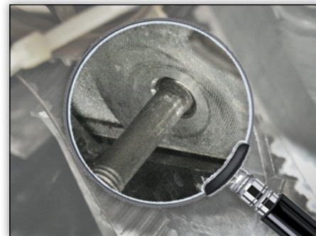
Fig. 2: De tapbout is correct ingeschroefd.
