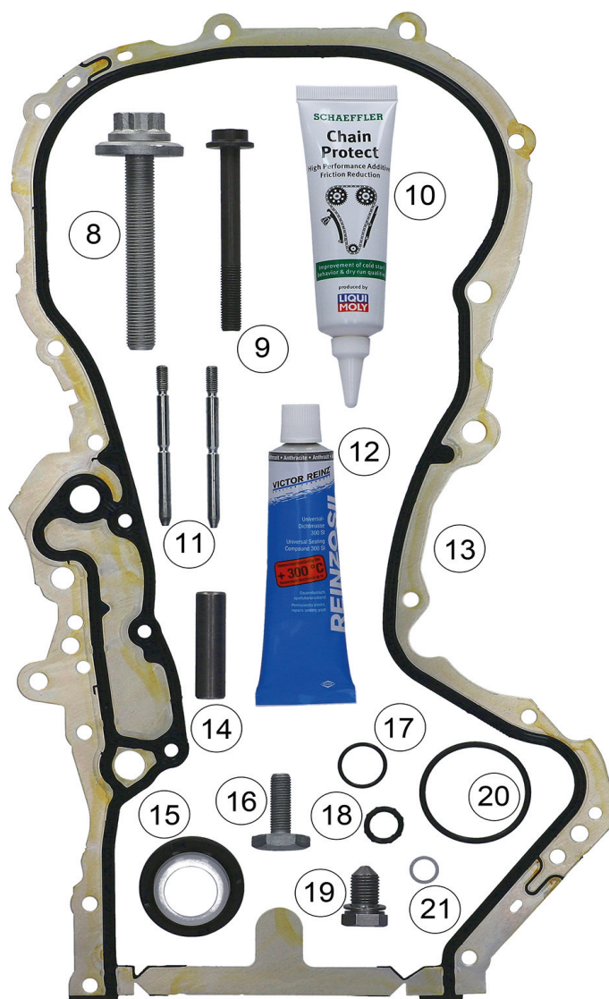
Figure 2: 559 0154 30/559 0154 31 - Timing chain KIT attachments
