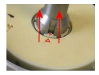
5) Pay attention at the new sensor: the spring clip has to be perfectly orthogonal to the plastic structure, in order to make both the sensor "disks" in-built.
