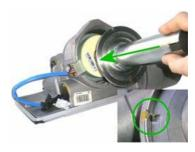
11) Insert the plug in its housing.
