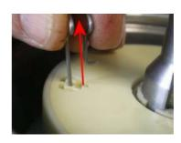
10) Reassemble hose, gasket and elastic ring.
