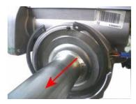
Align the reference signs, rotating the shaft if needed.
