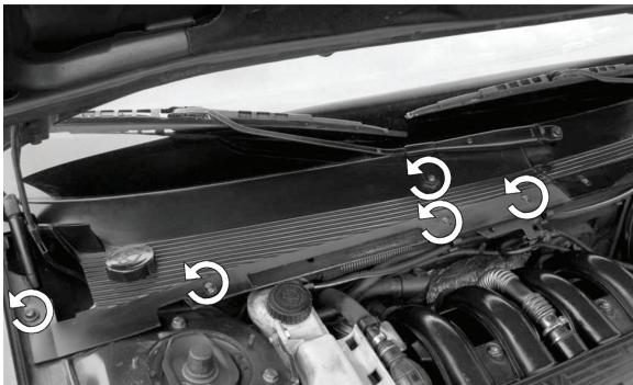
(EN) Loosen the screws of the cover under the windshield
