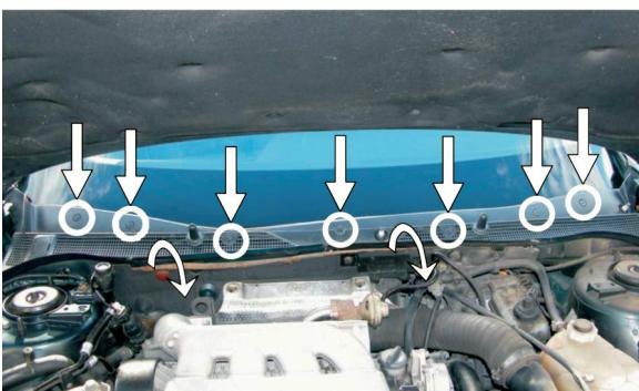
(EN) Loosen the screws of the screen under the windshield. Remove the segment of the screen under the windshield
