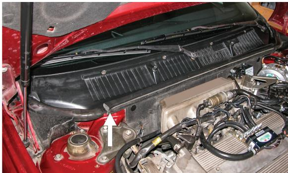
(EN) Remove the rubber seal
