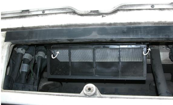
(EN) Open the locks and remove the filter seat
