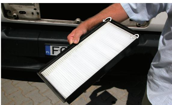
(EN) Remove the old filter from the seat, put the new one in and perform the opposite to all the previous actions in the reversed order
