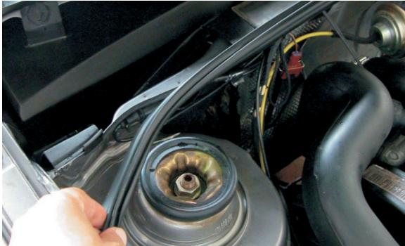
(EN) Remove the rubber seal
