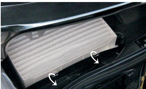
(EN) Unlatch the filter from its socket
