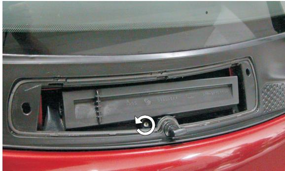
(EN) Loosen the screw and remove the cover of the filter
