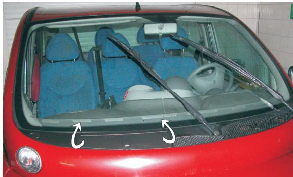
(EN) Move the wipers upwards and dismount the cover of the filter chamber
