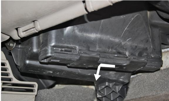
(EN) Remove the filter fastener, remove the old filter, insert the new one and carry out the opposite to all the previous operation in the reversed order
