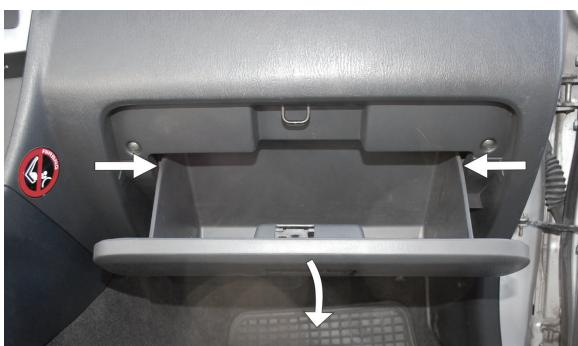
(EN) Remove the glove compartment
