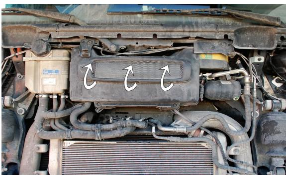
**(EN)** Detach the protection grid from the filter
