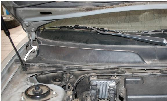
(EN) Remove the rubber seal
