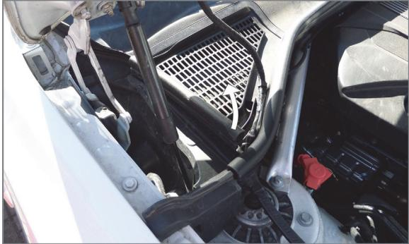
**EN** Remove the rubber seal
