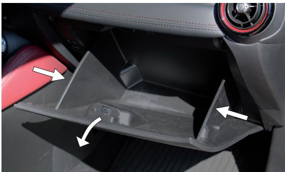
(EN) Open the glove compartment, the filter is located behind the rear wall of the compartment
