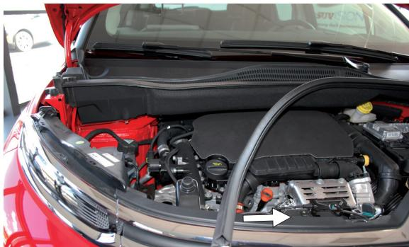
(EN) Remove the rubber seal
