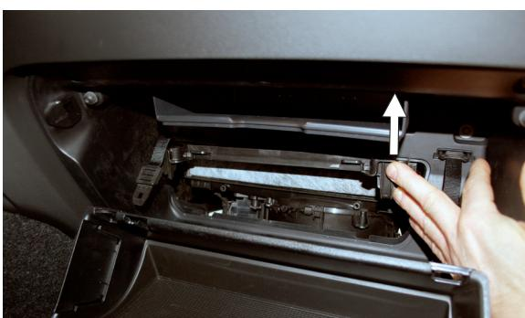
(EN) Carefully lift the cover of the filter
