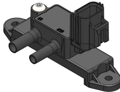
You will notice the design of the SMPE manufactured exhaust pressure sensor differs from the original unit. The OE design uses a ceramic capacitive device which is prone to early life failure and is less accurate than the modern electronic pressure sensor used in our re-designed unit. We were able to repackage the electronic sensor and attach it to a mounting bracket, ensuring the same footprint as the original design
