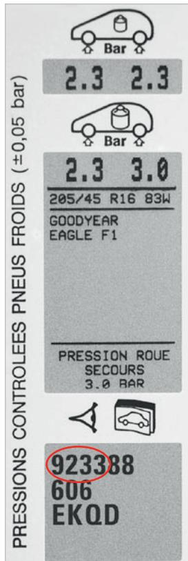
The RP number (Orga) is in the bottom half of the vehicle data label. The last two digits of the number are irrelevant as far as looking for the spare part is concerned.
