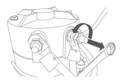
**3.3** The electric motor can be used as a pump or traction motor, depending on the application. In either case, undo the fixing bolts and remove the electric motor from the pump or transmission. Follow the machine or system manufacturer's instructions.
