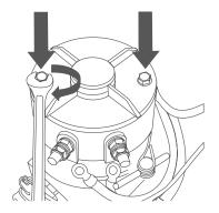
**3.8** Connect the electrical cables to the electric motor. Take care to route the cables properly, making sure that the cables do not come into contact with hot or abrasive surfaces.
