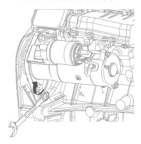
3.8 Connect the starter motor. Make sure to connect all cables to the associated terminals. Take care to route the cables properly, making sure that the cables do not come into contact with hot or abrasive surfaces. **3.9** Connect the battery leads to the battery. First connect the positive lead, then the negative lead.
