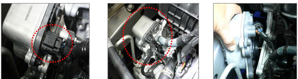
7. Install the new water pump, insert the connector until click, and install the air cleaner.
