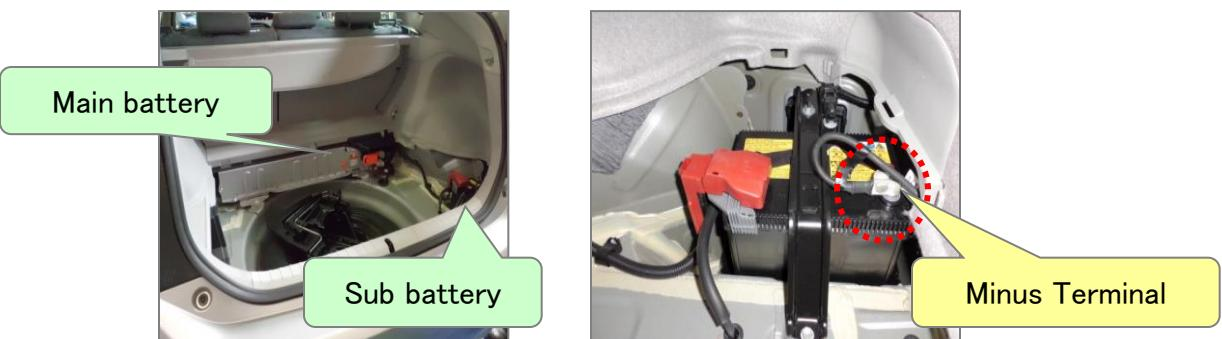
2.Remove the “Service Plug” of the main battery.
