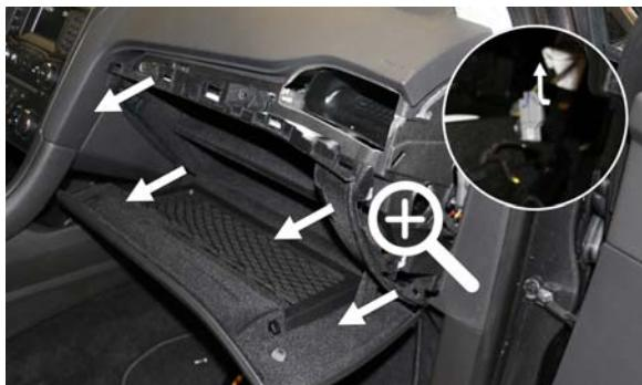
EN Remove the glove compartment, disconnect the electric circuit
