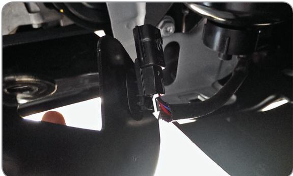
**(EN)** Disconnect the electric circuit
