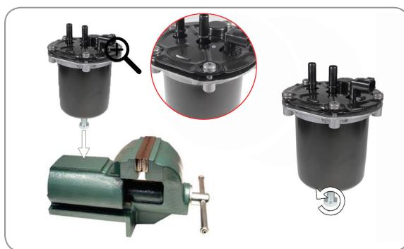
(EN) Hit vigorously so that the filter cover loosens and remove the screw
