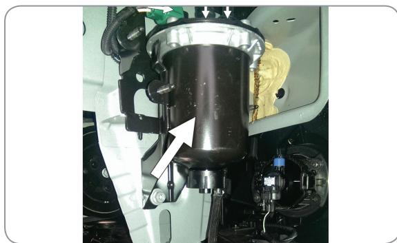
**(EN)** Replace the filter in the vehicle, plug the fuel lines and mount the wheel arch and wheel
