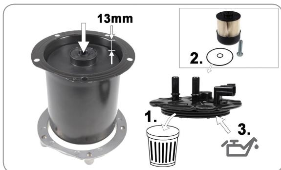
**(EN)** Install the new filter to a depth of 13 mm. Remember to replace the seals
