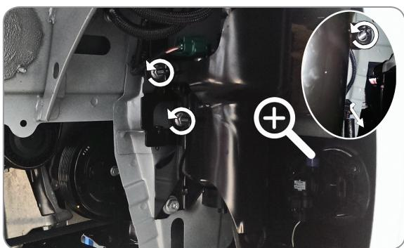
EN Loosen the screws of the filter housing
