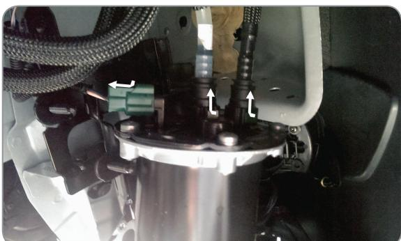
**(EN)** Disconnect the quick connects of fuel filter pipes, disconnect the electric circuit
