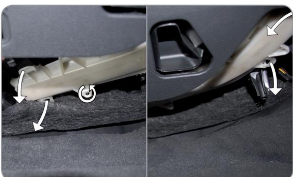
EN Loosen the screw of the filter housing
