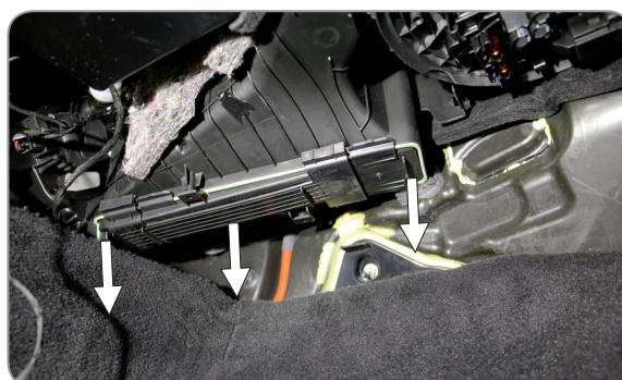
**(EN)** Remove the cover from the filter chamber
