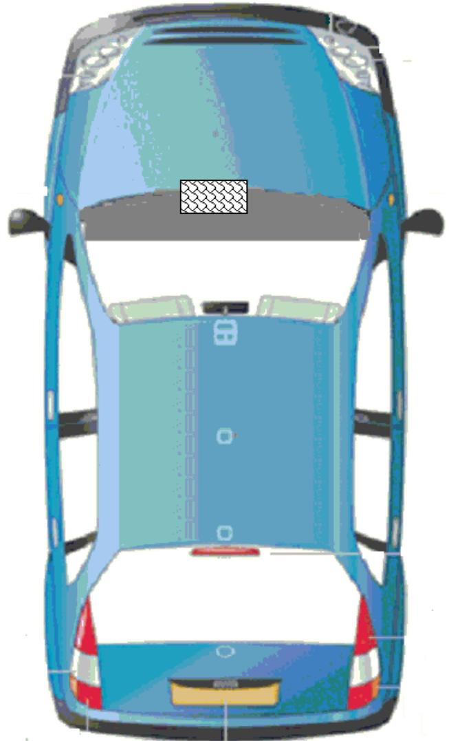
1. The Cabin Filter is located centrally in the engine compartment at the base of the windscreen.
