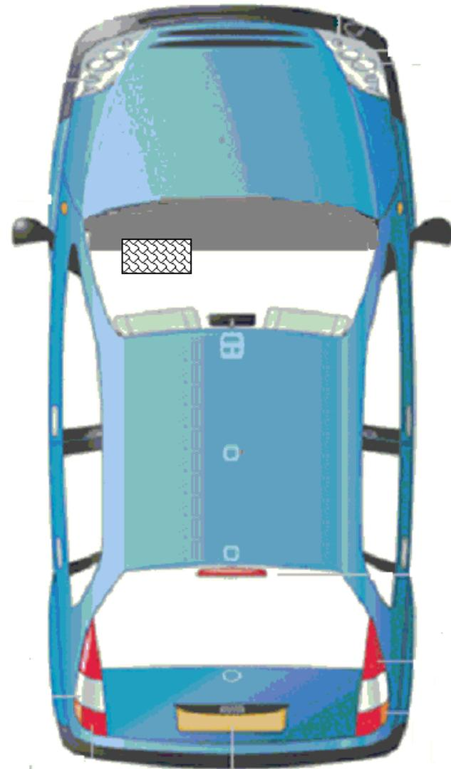
1. The filter is located behind the glove compartment.
