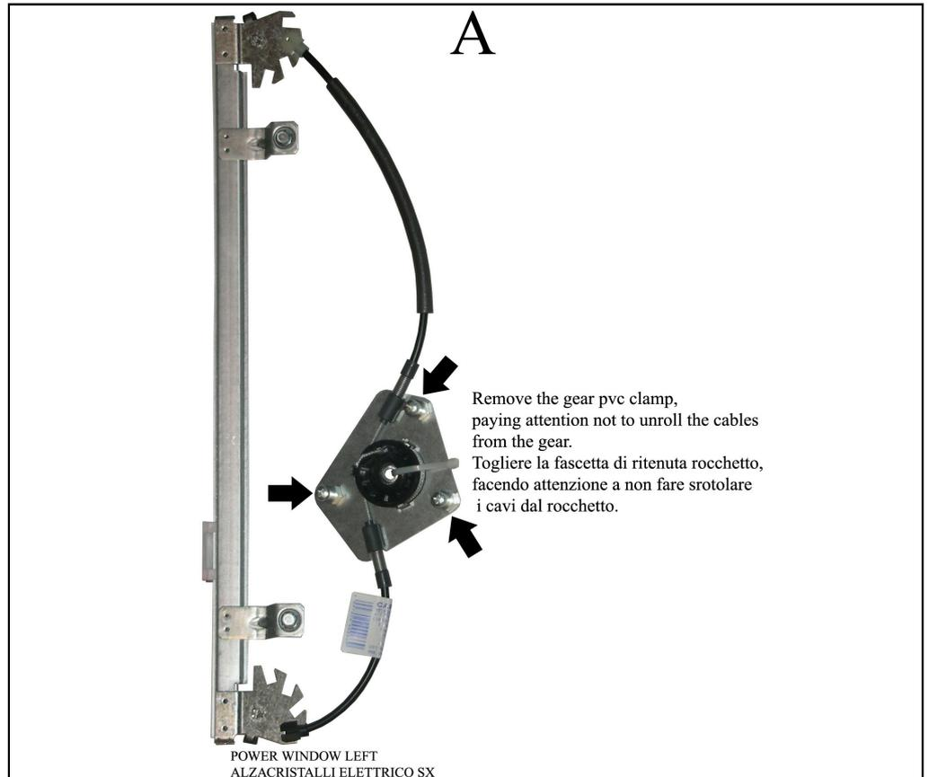
Remove the gear pvc clamp,
