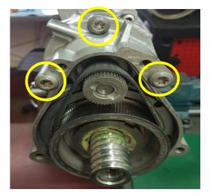
9. Using a screw driver turn the washer and black plastic bearing in a clockwise rotation until the belt is tight.
