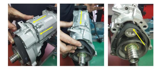
8. Screw the motor in position.
