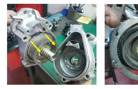
4. To start assembling the motor, carefully position the black plastic bearing. The position of the notch should be parallel with the housing as shown below. Please note this bearing will only move in an anti-clockwise rotation.
