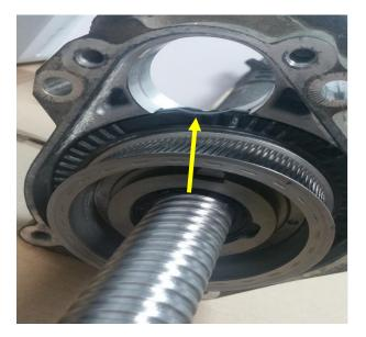
5. Re install the washer. The washer must be positioned to match the same notch as the black plastic bearing.
