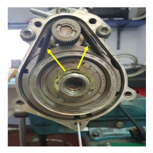
10. Place the locking pin in position and gently tap to lock the washer and black plastic bearing into position. \*\*<u>check there is sufficient clearance between the teeth of the motor and the washer</u>\*\*
