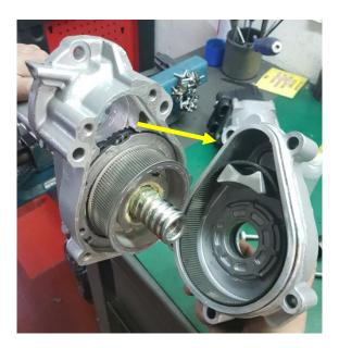
2. Carefully remove the belt from the inside of the housing, and keep safe for later use.
