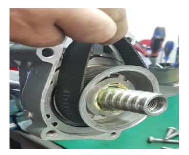
7. Hold the belt and insert the motor through the housing. Slide the belt over the teeth on the motor.
