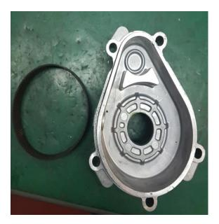
3. Carefully remove the washer, and keep safe for later use.
