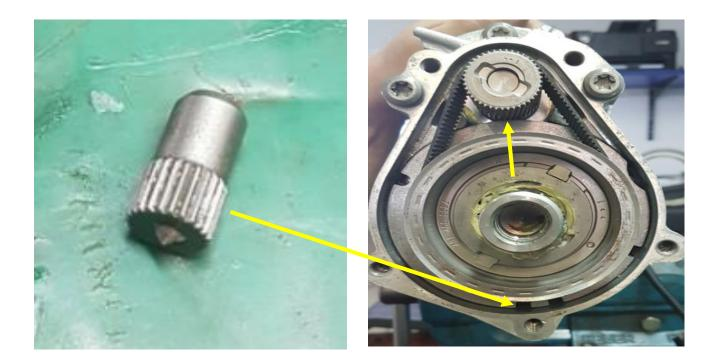
11. Re install the housing, and secure in place with 5 screws
