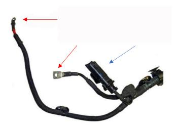
ERRM2077 is equipped with 2 Plug connectors (Blue Arrows) and 1 Spade connector as below (Red Arrows).
