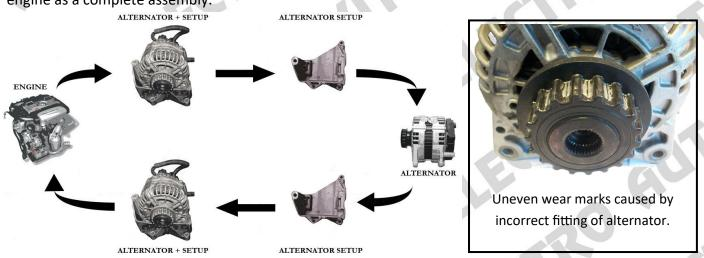
If this is not done in the correct way then it will result in the 'Eurogrip coupling / Cog belt' not being aligned correctly and becoming worn and also causing the clutch pulley to fail.
