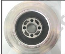
Picture of a new TVD. The dampening insert is in one piece with no cracks or imperfections.
