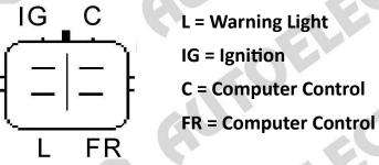
If there is no signal to the 'C' terminal on the alternator from the ECU the alternator will show overcharge at around 15.7V. This would indicate either a wiring break in the loom, the connector pins in the plug are damaged or open too far to make connection or the ECU may be at fault.
